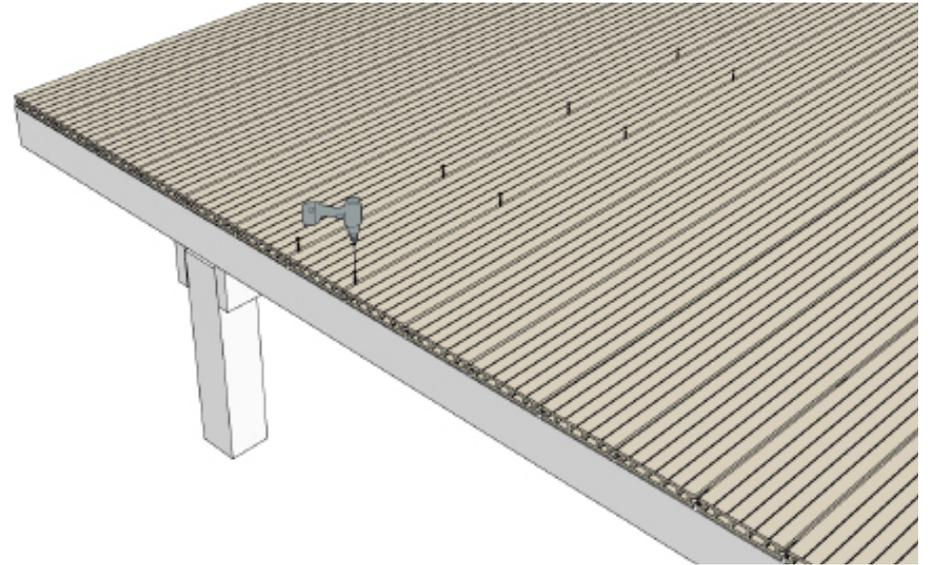
BB Then slide all the T-Clips out of the board.
