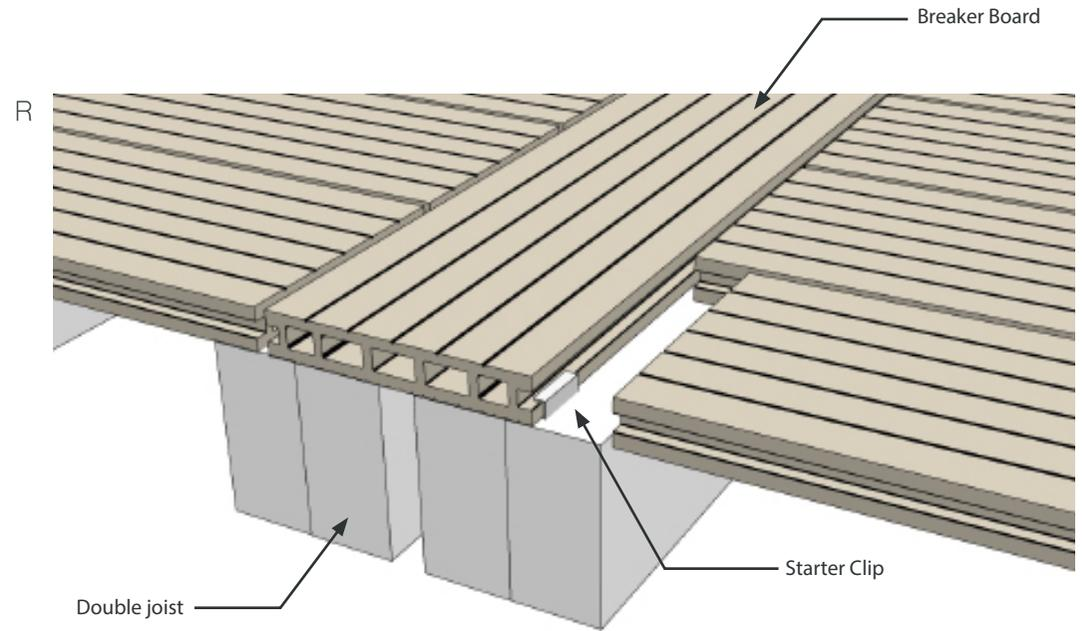
Breaker Board - Starter Clip - Plan View
