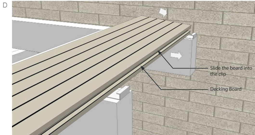
E Ensure the board is fully installed into the clip before proceeding.
