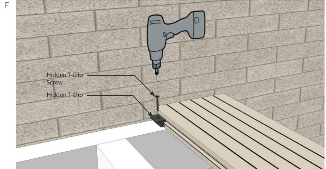
G Install the remaining T-Clips part way as above. One T-Clip should be installed per joist.
