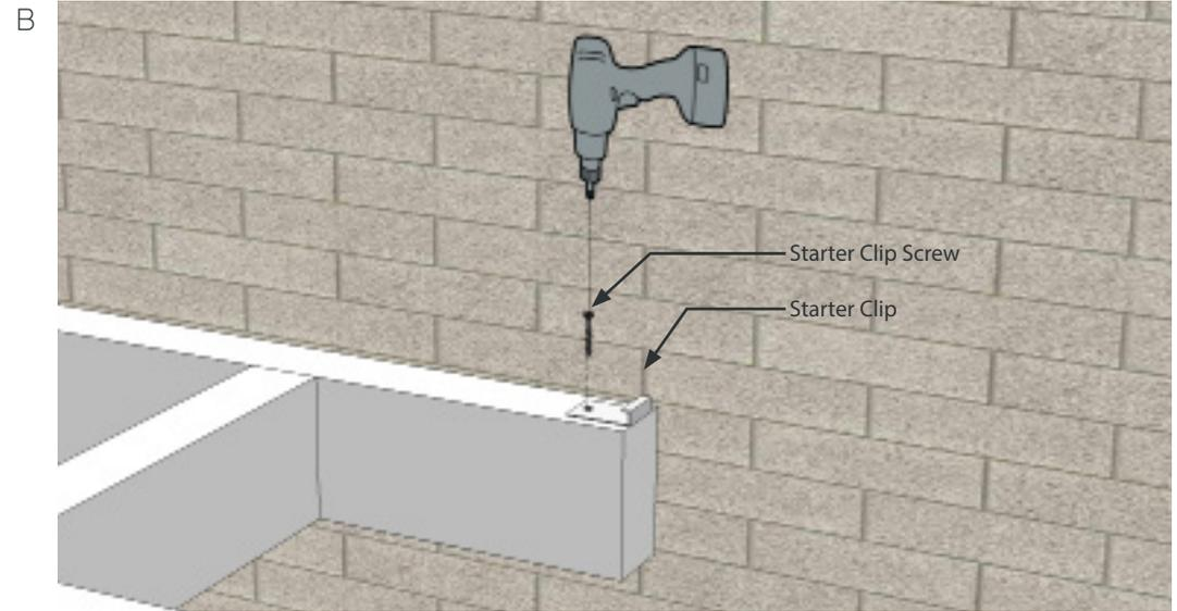
C Using a deck board or string line install the remaining starter clips, taking care to ensure they are aligned
