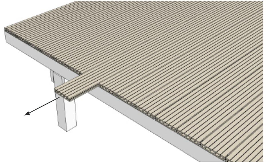
DD The new board can now be inserted. Take the opportunity to check the sub frame for any damage / wear.
