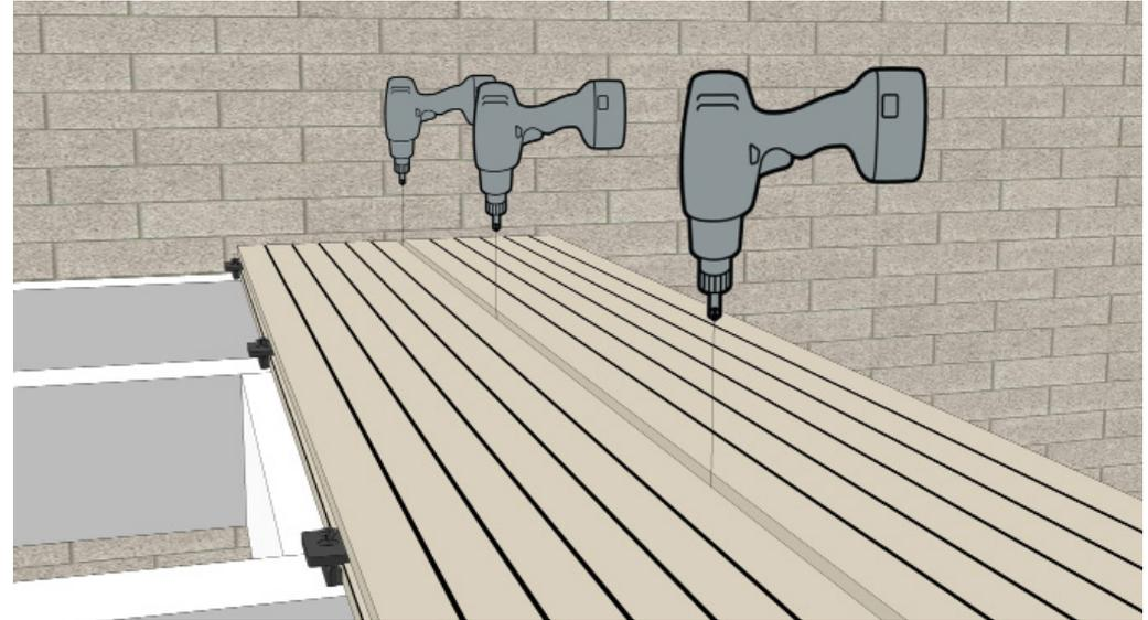
L When Installing the T-Clips Take care to use a screw bit of a suitable width to avoid damage to the boards.
