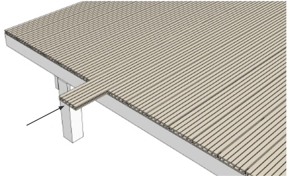
Then slide all the T-Clips back into the grooves of the board, and back into their original positions.
